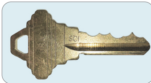
Figure 10-34: A successfully impressed Schlage key
