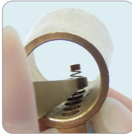
Figure 5-21: Inserting a spring into the bible
