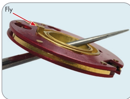
Figure 12-17: Wheel 3, the one closest to the drive cam, always has a protruding fly, while all the other flies are flush with the wheel.
