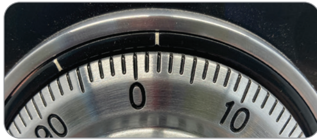
Figure 13-12: Notice that the reading has shifted slightly right when the fence slips into the gate.
