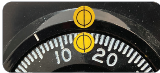
Figure 12-11: Fine-Line dial indicators by Taylor Technologies highlight subtle changes and can make all the difference in your search for clues.
