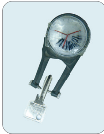
Figure 9-18: Kroeplin calipers with marker lines added to the dial for quick reference of ABUS cut depths
