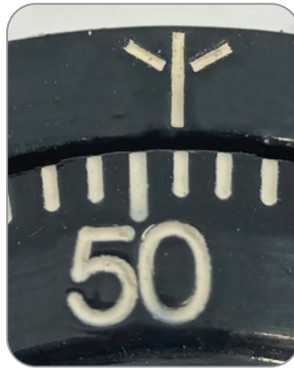
Figure 13-5: A reading just under 51
