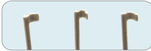
Figure 6-14: Different dimple pick tip shapes
