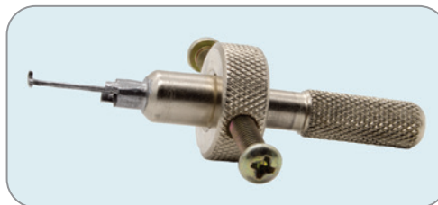
Figure 7-33: Homemade tool to pick a DOM Diamant
