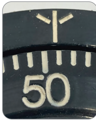
Figure 13-6: A reading of 50.75 or possibly 50.8, depending on your individual calibration
