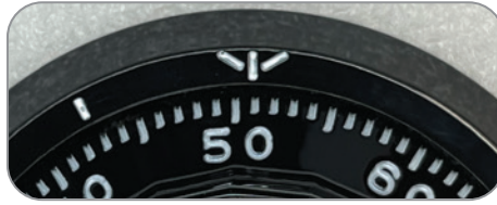
Figure 14-6: Here the index lines are slightly overlapping, which constitutes a reading of 50 Next Overlap.
