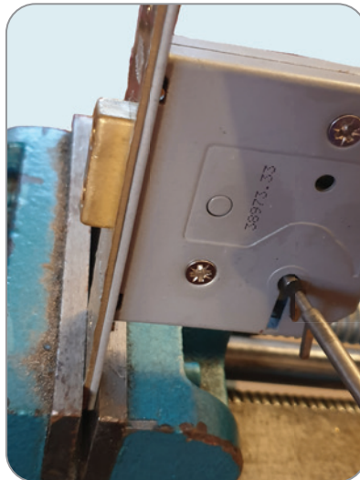
Figure 15-21: Using a 2-in-1 to pick a three-lever UNION lock
