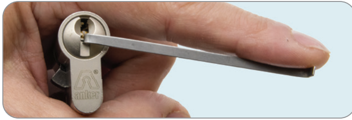
Figure 7-3: Tensioning at the center of the plug
