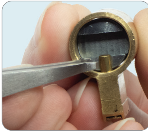
Figure 5-19: Releasing a driver pin
