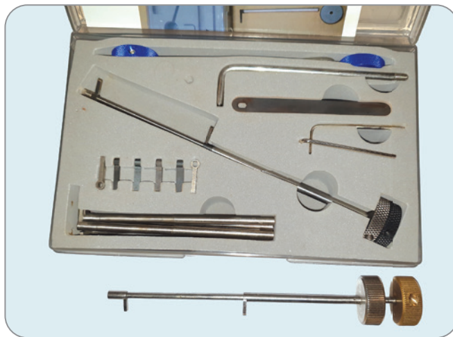
Figure 15-19: Seven-gauge 2-in-1 picks used to open non-curtained, pin-type locks with all levers on one side of the bolt
