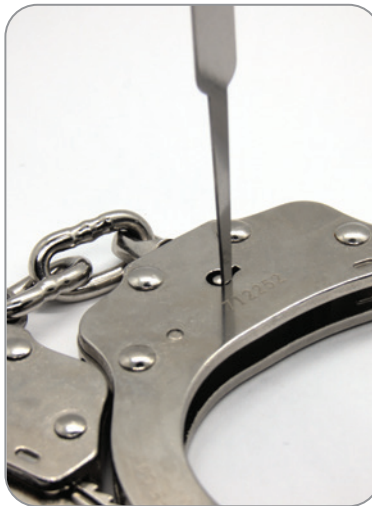
Figure A-15: Rotate the picking tool clockwise to release the double lock, and counterclockwise to retract the pawl
