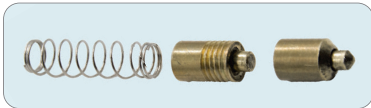
Figure 4-12: One pin-in-pin stack from a Mul-T-Lock; from left to right: the spring, inner and outer driver pins, and inner and outer key pins
