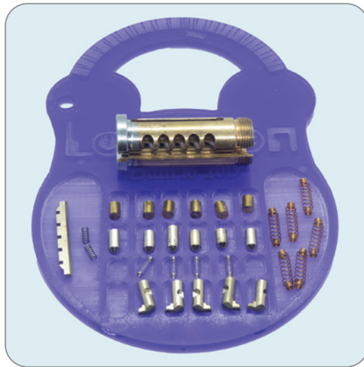
Figure 4-4: A disassembled Schlage Primus showing the bottom of the plug, where the five side pins are inserted
