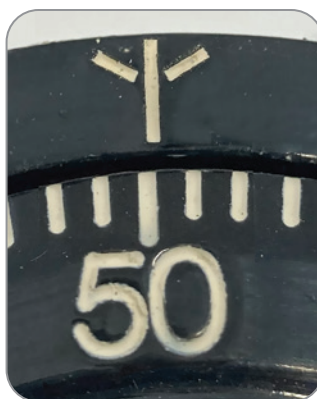
Figure 13-7: Is this reading still 50, or have you made it to 50.25 (or in tenths, 50.1 or 50.2)?
