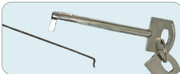
Figure 15-26: A homemade Hobbs pick (cut-down key and wire) for the Chinese safe lock shown in Figure 15-25
