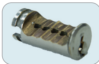
Figure 10-35: A filed-down ABUS plug
