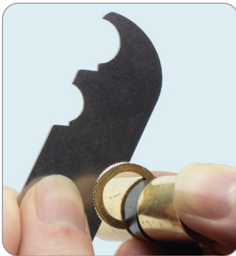
Figure 5-26: Reinstalling a C-clip using the SPARROWS Gut Wrench
