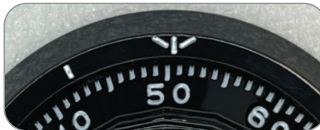
Figure 14-4: The opening index appears between 50 and 51, so you'd call this 50 Middle.
