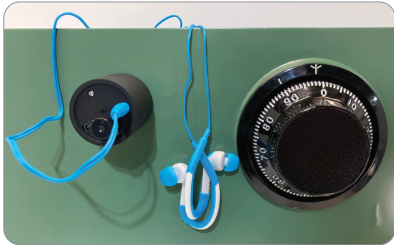
Figure 12-5: This old filing cabinet drawer has been turned into a dialing station—not particularly handy to carry around, but the EZ AMP attaches to this solid metal surface magnetically.
