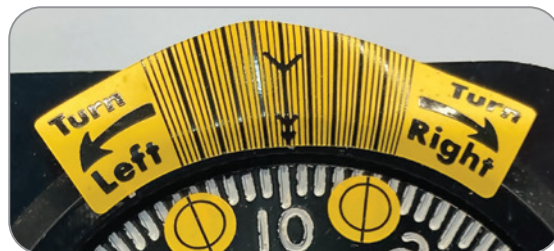
Figure 12-12: Lockmasters Read Eze stickers help define the increments between these blurry lines.
