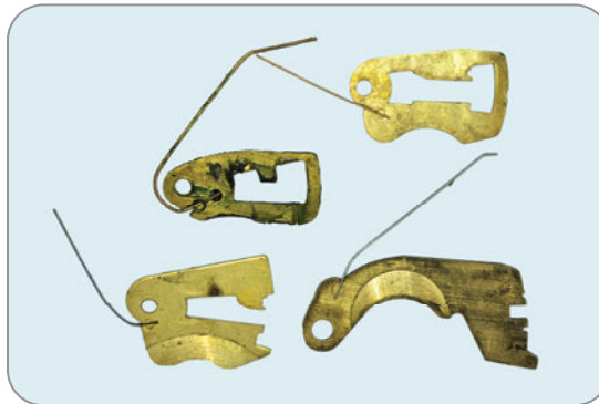
Figure 15-7: Clockwise from bottom right: a Chubb 110 detainer, an ICL/MAX6MUM detainer, a lever from a random three-lever lock, and an unused lever from a prototype lock
