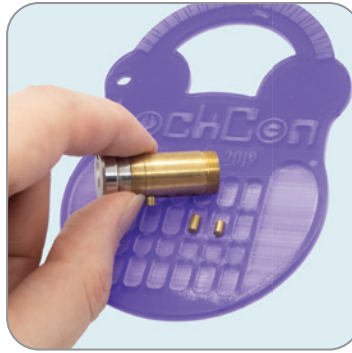
Figure 5-18: Dumping the key pins from the plug
