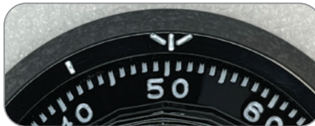
Figure 14-3: Because the edges of the opening and number index align, this reading is considered 50 Aligned.
