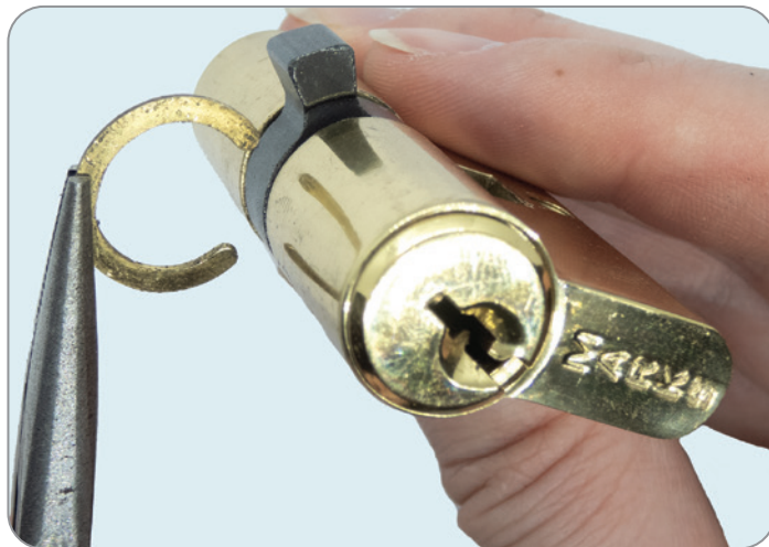
Figure 5-13: Removing a loosened C-clip with pliers
