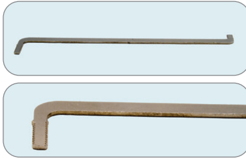
Figure 6-4: A flat, serrated tension wrench
