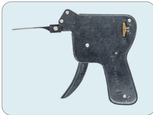
Figure 6-18: A manual pick gun that fires only upward
