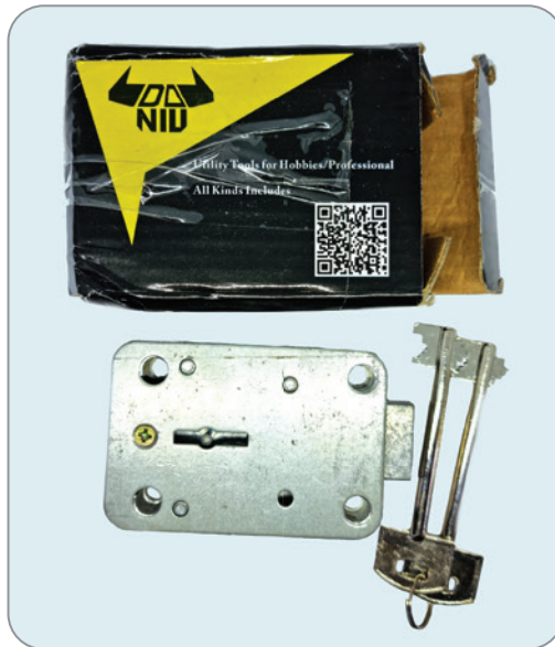
Figure 15-25: A cheap, double-bitted safe lock from China. Note the drill pin in the center of the keyway.
