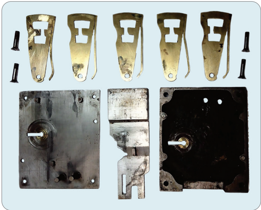
Figure 16-7: This Ratner Safes lock is the very model of simplicity; shown here are the two halves of the case, the bolt, five levers, and four screws to hold it together. Image courtesy of autom8on (@a8n_pub), © 2021 by Stephen Wilson.
